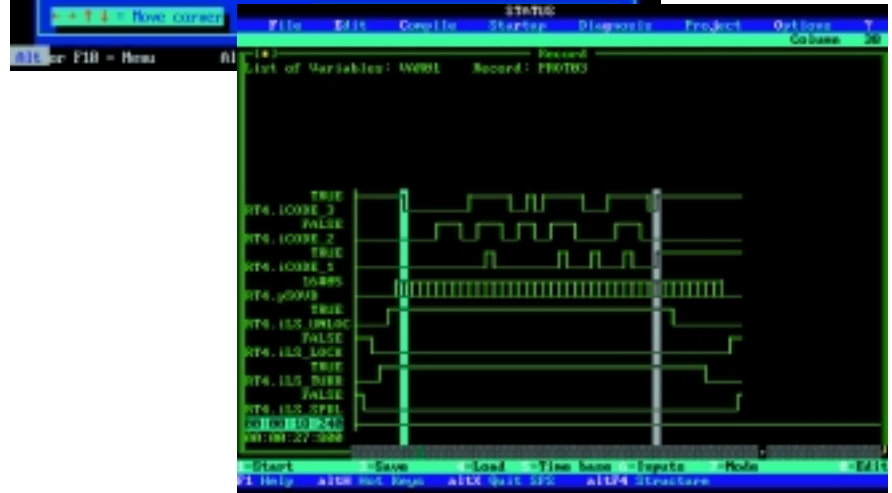
PLC logic timing analysis using the PLC logic analyzer
