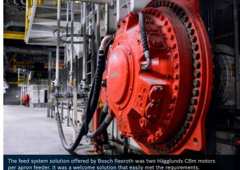
based on two motors that share the load on each feed unit, with a capacity of 8,000 tons per hour, a variable speed of 0–7.46 rpm and a starting torque of
