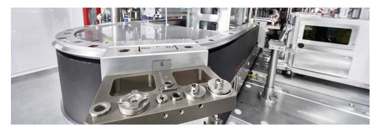
ActiveMover from Rexroth ensures short auxiliary process times in a Behr Systems assembly system
