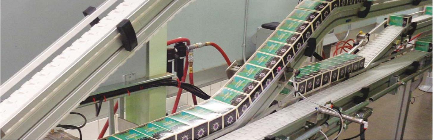
Modern tea bag production with the flexible conveyor system VarioFlow *plus* from Rexroth
