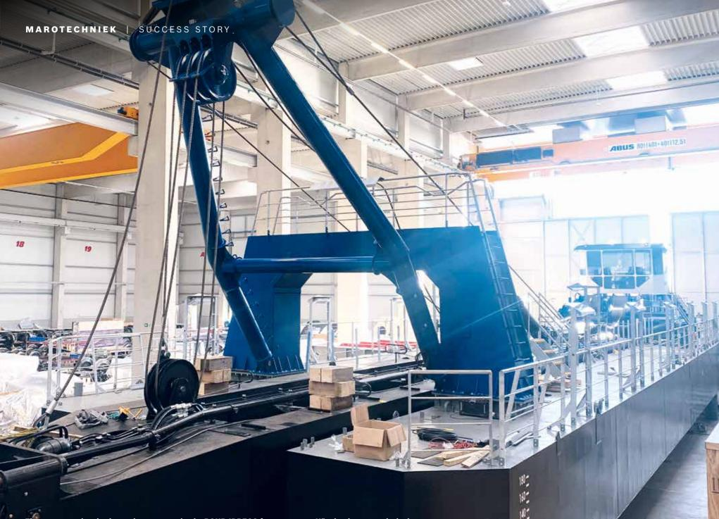
The cutter-suction dredge under construction by ROHR-IDRECO features seven Hägglunds-powered winches.
