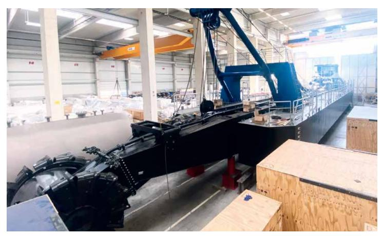
The dredge has a maximum output of 270 cubic meters per hour.
